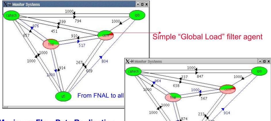
Maximum Flow Data Replication Path Agent Deployed to each RC and evaluates the best path for real-time data replication
