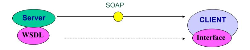
The client can dynamically generate the data structures and the interfaces for using remote objects based on WSDL
